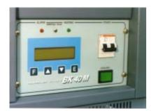
The BK40 M temperature calibrator is an instrument used to calibrate transducers, RTD and temperature-measuring sensors in the laboratory. The possibility to generate positive and negative temperature ramps makes it suitable for use in calibrating and testing thermostats.
